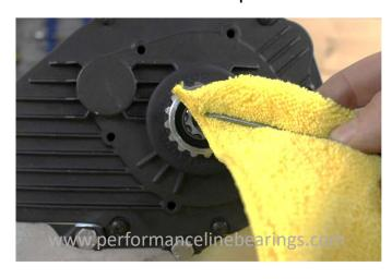
Step 3, Apply a thin film of silicone or water resistant grease
