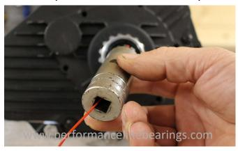
Step 6, The wire is to let the air escape as the seal is pushed in. If you don't have the crankshaft fitted, this step is not necessary.
