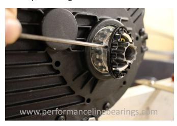
Step 2, Apply Bosch bearing protection long life tacky grease.
