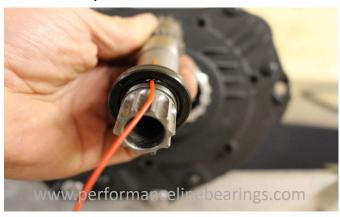
Step 8, With the seal in place past the circlip grove, the wire can be pulled free. Push the seal once more to ensure it is fully seated.
