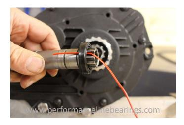
Step 7, Ensure the tool you use fits over the crankshaft all the way down to the bearing. Pass the wire through the tool and push the seal until it stops at the bearing.
