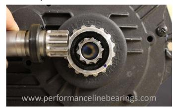
Step 9, Re-fit the crankshaft outer circlip.
